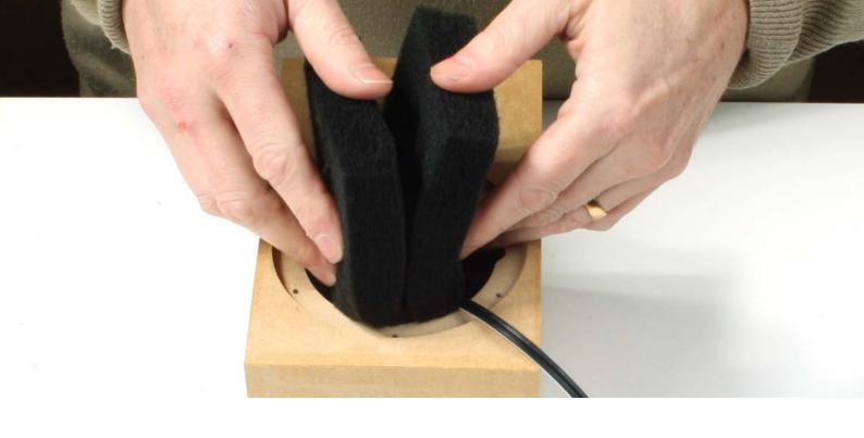
Before inserting the acoustic lining, cut an opening in the shape of a cross with a sharp blade. The cross should be centred 205mm from the top end.
