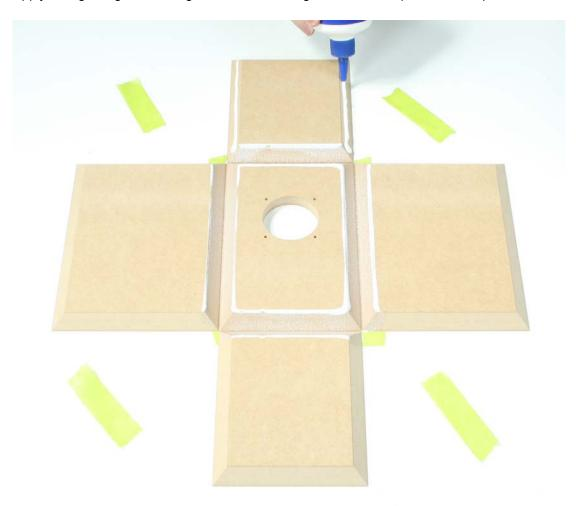
Lift up the panels and hold together with pressure, securing them in position with masking tape. Apply the masking tape with firm pressure so that the panels are held together with moderate pressure.
