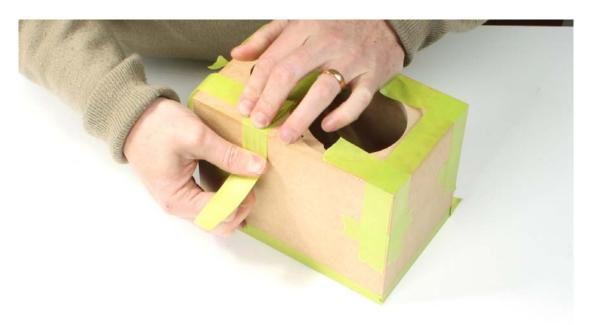
All joints should be covered. If pressure is applied when taping, no further clamping is required.
