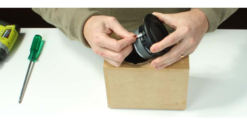
It's now time to install the driver. Push the connectors onto the driver tabs. Correct polarity is important but this is made easy by using faston connectors that are sized to avoid mistakes. The larger negative connector goes to positive and the smaller negative connector goes to the other. Avoid excessive force, which can damage terminals. If you find the fit is tight, you can use a small flat head screwdriver to open them out slightly.
