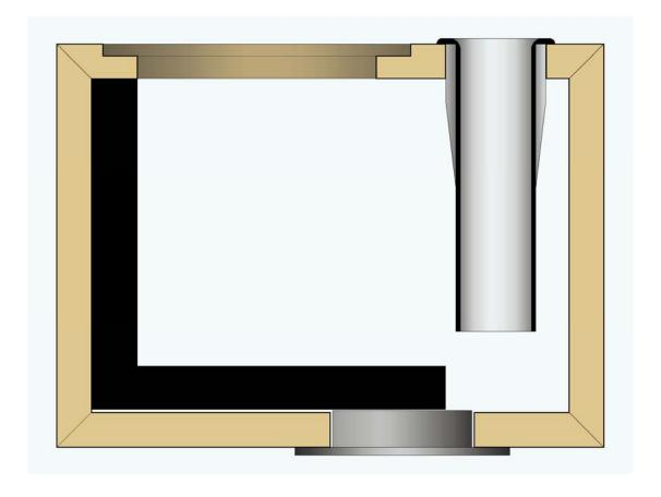
Note: the clearance around the port is essential to retain the correct tuning.
