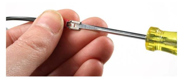
Screw in the terminals with the wire loom already attached.
