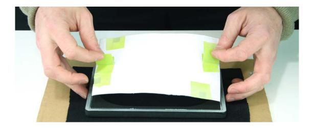
Glue is only required on the back surface as shown here – no glue is required to the sides.
