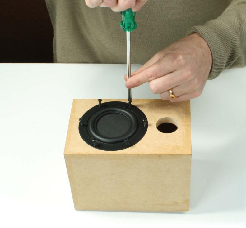
Screw the driver into place with a Phillips head screwdriver, securing the shaft with the other hand. Pushing the port into place completes the assembly. Your new kit is now ready to rock!
