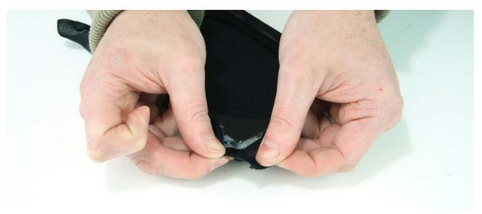
Hold the cloth with both hands, then pull it back over the frame. Stretch it firmly, pulling back into the correct position. After stretching it into place, press down to the glue area.
