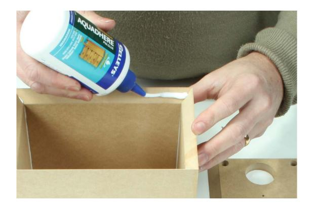
Note: the orientation of the front baffle is determined in the next step. Before gluing the baffle in place, please check the instructions carefully.
