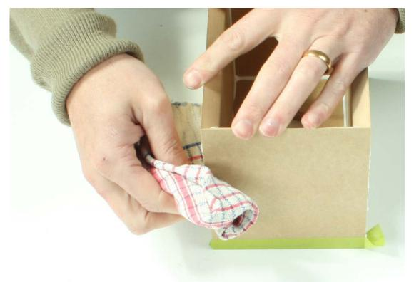
Apply a thick glue bead around the internal surfaces of the mitres. You may prefer a zig zag pattern with a thinner bead. It's a good idea to remove the panel and confirm even coverage.
