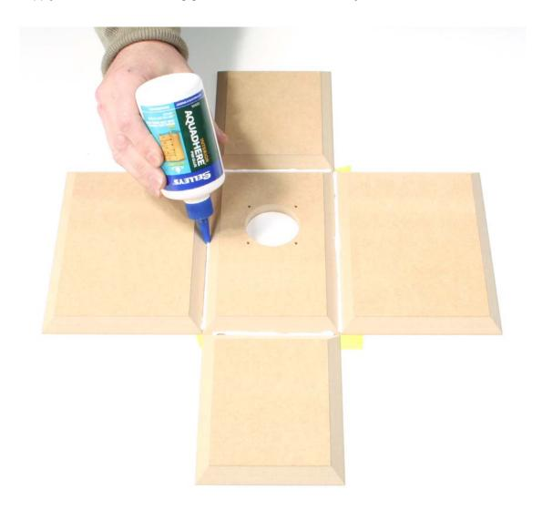
Apply a second bead. Since the glue will tend to run down towards the bottom, it's a good idea to apply the glue above half way up to ensure even coverage.
