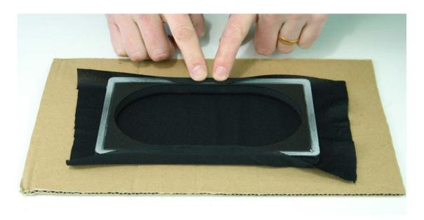
Now press the cloth onto the glue on the back of the frame. Start with one side and then follow with the opposing side, stretching the cloth. When stretched with adequate tension, you will see ripples in the fabric between the two points of contact on the frame. These will be stretched out when the cloth is attached to all sides of the frame. Without adequate tension, the grille cloth may tend to sag. Too much tension applies undue stress on the glue holding the fabric in place.
