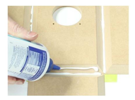
Confirm the amount of glue applied by folding up the first panel. The glue should cover the entire surface in contact. It's preferable to see the glue ooze beyond the join slightly. This provides visual feedback on whether the glue has set. Once set, PVA glue becomes transparent.
