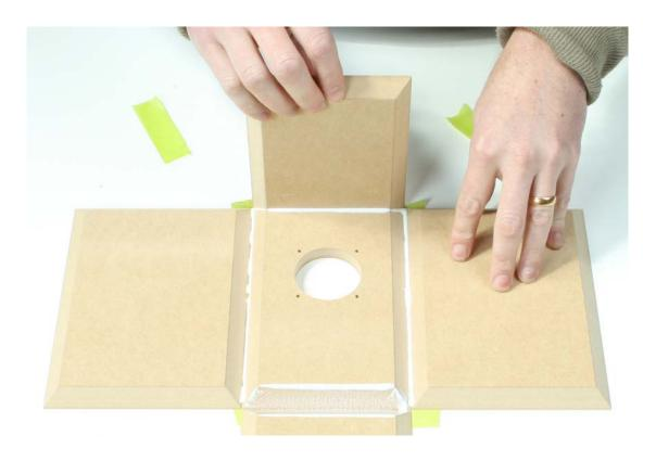
Apply a single larger bead of glue to the remaining sides on the top and bottom panels.
