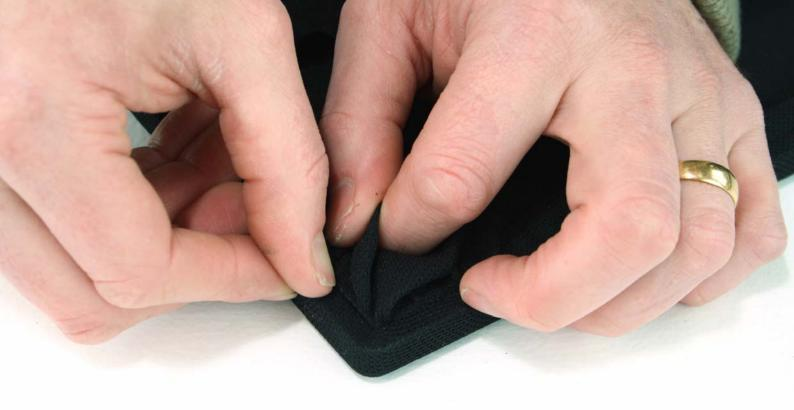
Now you can use your thumbnail to find the cut line. Pressing your nail into the trench, score all the way around. Then with a sharp blade, slowly and carefully cut away the grille cloth, using the trench as a guide.
