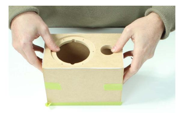
Wipe off any excess glue at the join. Then apply tape with tension to firmly hold the baffle in place. Tape should first be applied perpendicular to the join.
